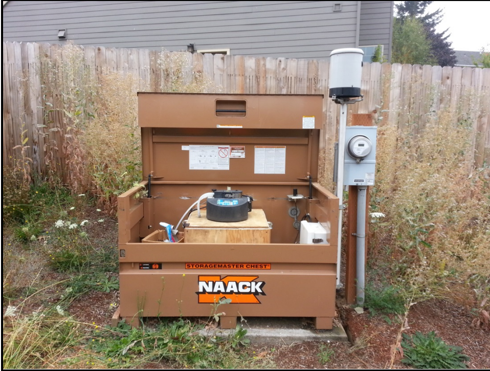
Figure 3 High density residential (HDR) site secure monitoring station equipment box and rain gage
